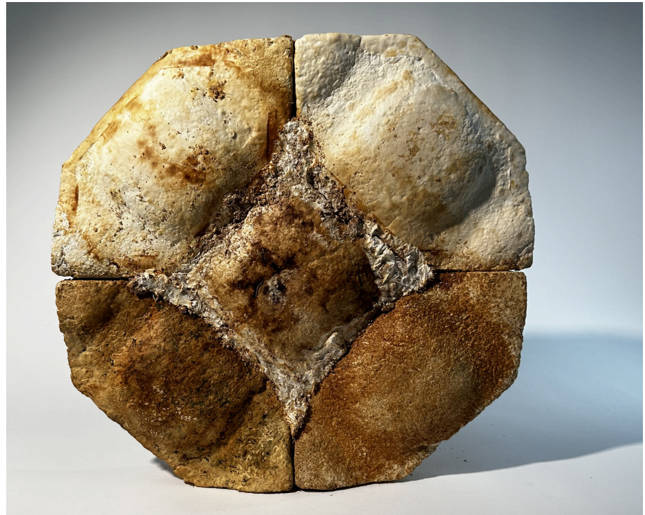
MULTI-DENSITY MYCO-BLOCK, FINISHED
