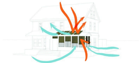
SUMMER DAY: HOT AIR EXITS HIGH WHILE COOL AIR IS DRAWN IN LOW
