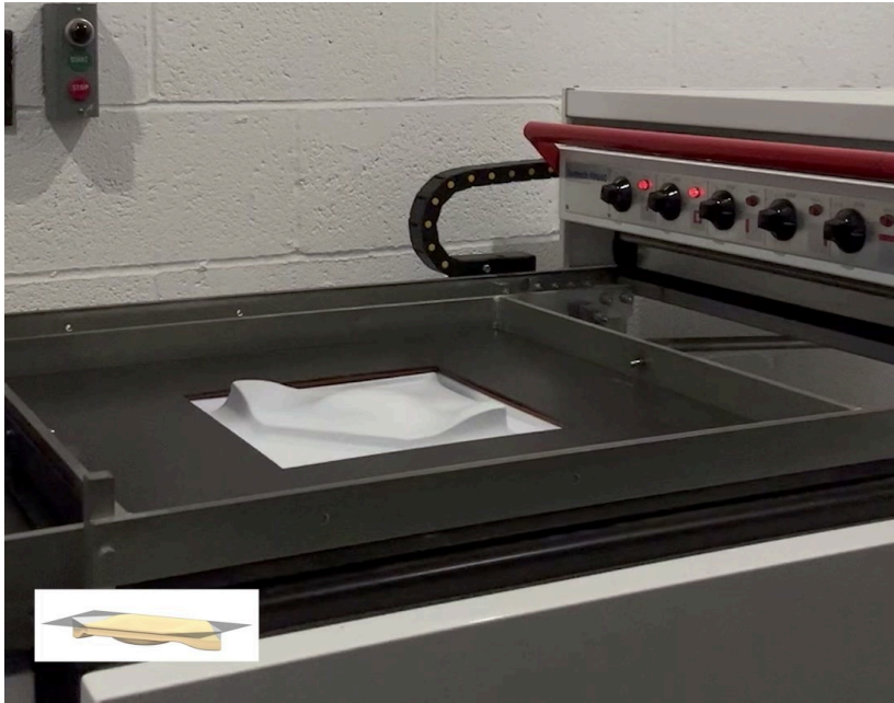
VACUUM FORMING THE MOLD
